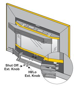
Slide the SIT valve extension knobs onto the valve knobs. Match the correct ext. knob with the valve knob.
